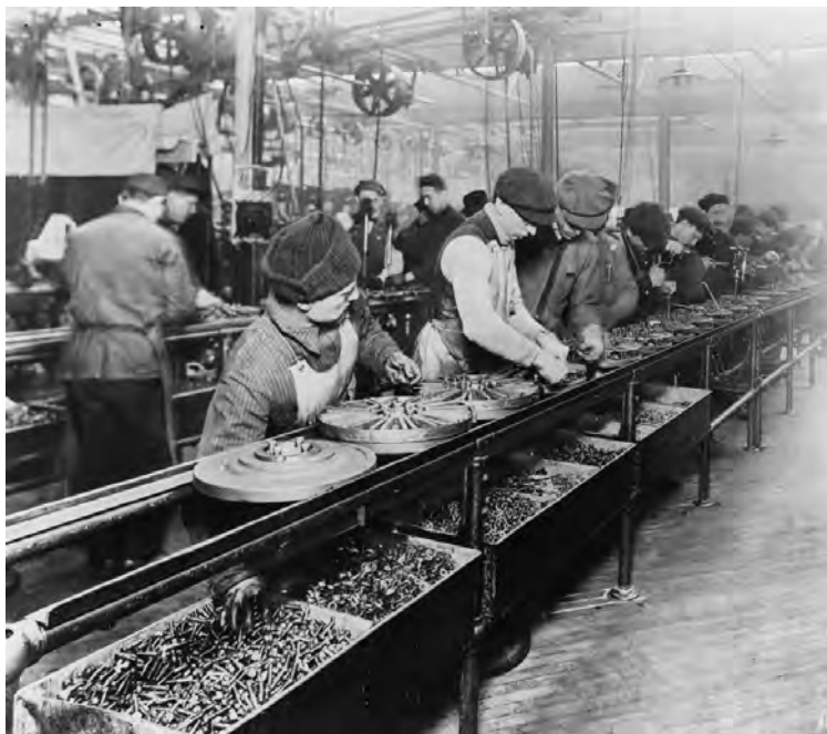
Figure 4.3 The First Assembly Line in the Automobile Industry was Implemented by Henry Ford.
